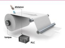
Torque regulation with pneumatic/electromagnetic brake and PLC
