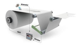
Regulation in torque with load cells or dancer roller
